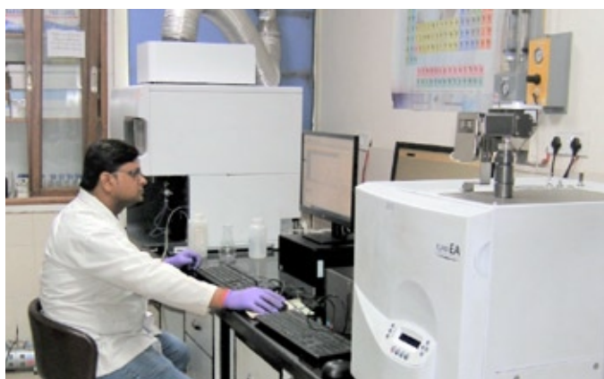
▲ Instrumentation for nutrient analysis by ICP-OES and CHNS Analyzer in IARI's Division of Plant Physiology.
