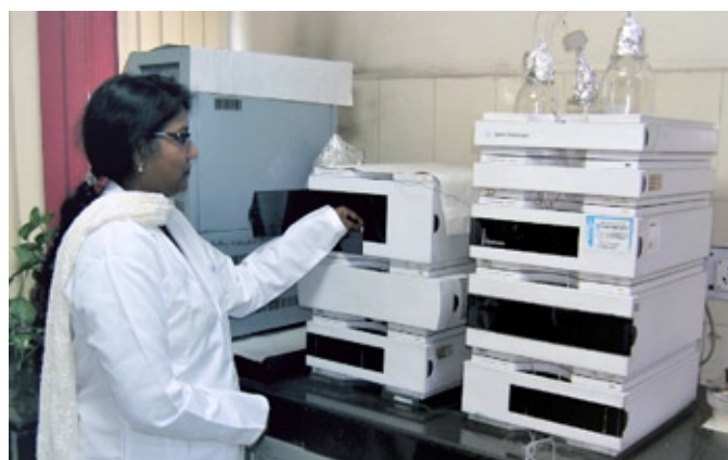
▲ Metabolite (amino acid) analysis by HPLC in the Division of Plant Physiology, IARI, New Delhi, India.
