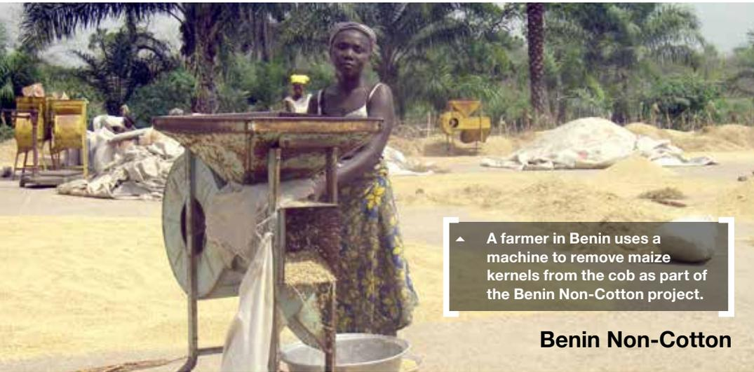
▲ A farmer in Benin uses a machine to remove maize kernels from the cob as part of the Benin Non-Cotton project.
